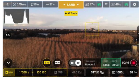
Exposure is locked on a building on the horizon: shutter speed is set at 1/500 s
